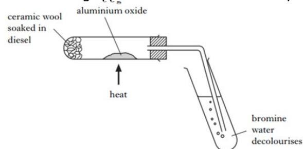
The aluminium oxide is a catalyst in this reaction.
